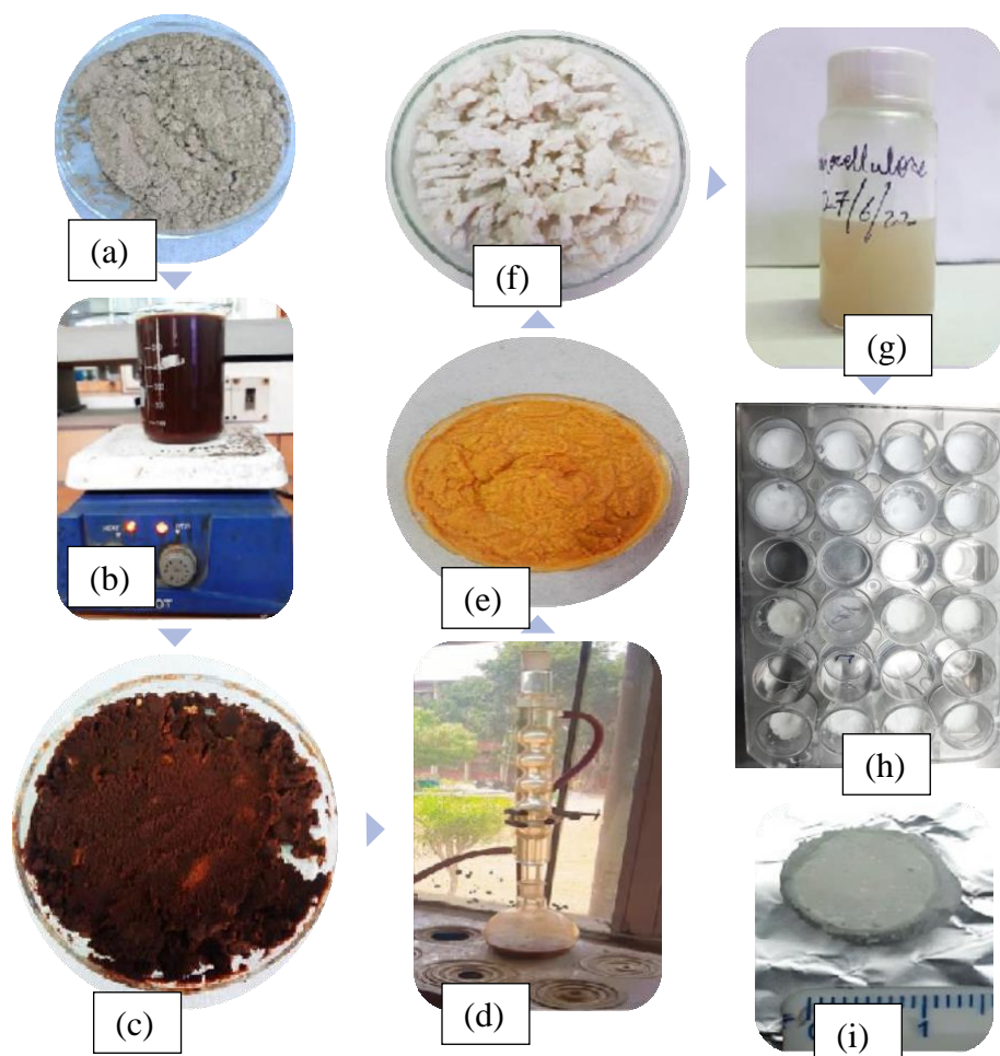
Fig. 1: (a) Groundnut shell powder, (b) NaOH treatment, (c) Delignified powder, (d) acid reflux, (e) acid refluxed powder, (f) bleached cellulose, (g) CNC, (h) fabricated and (i) freeze dried scaffold.
