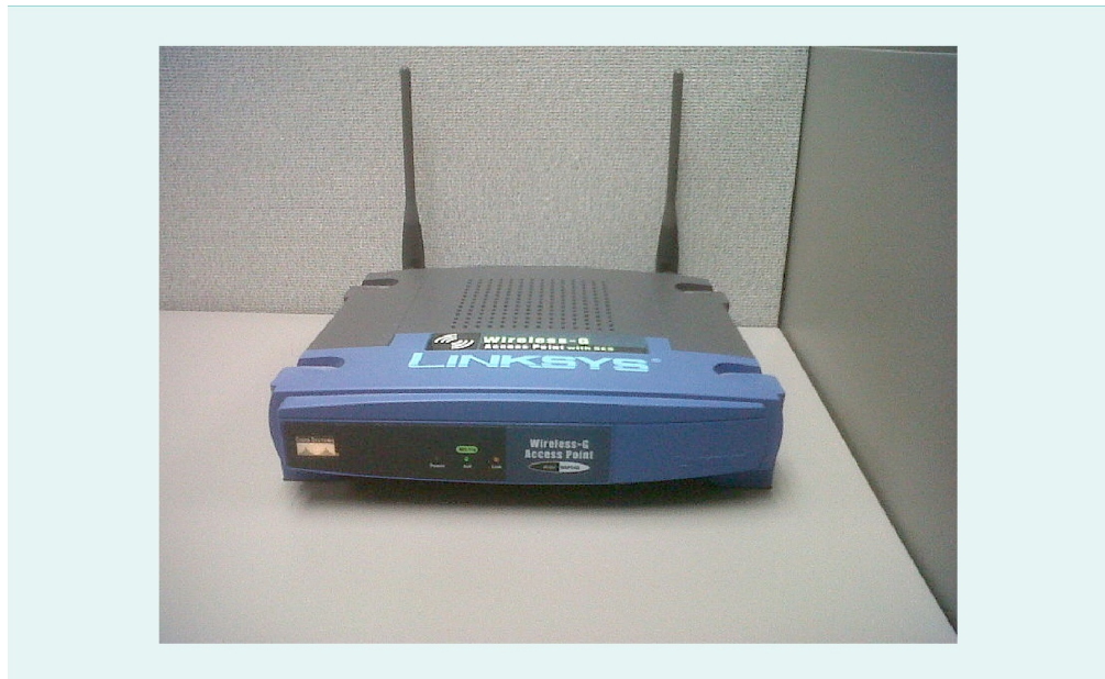
Figure 59: Wireless Access Point
