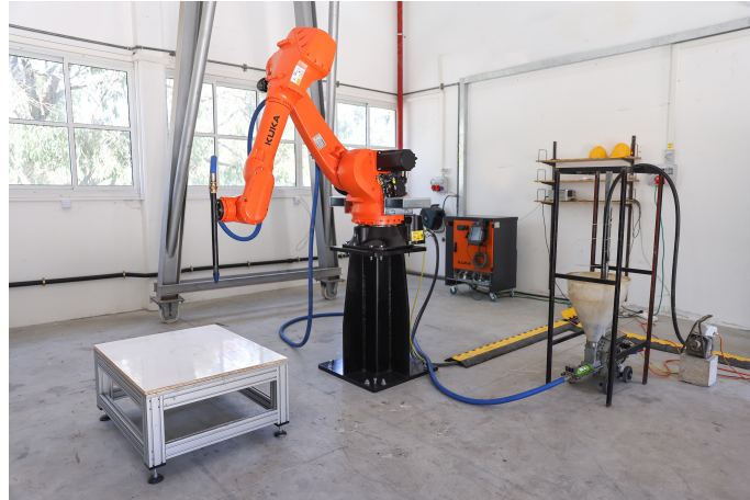
Figure 4: Setup of robotic cell for 3D printing of clayey soils, featuring an industrial robotic arm, mortar pump, and concrete vibrator.
