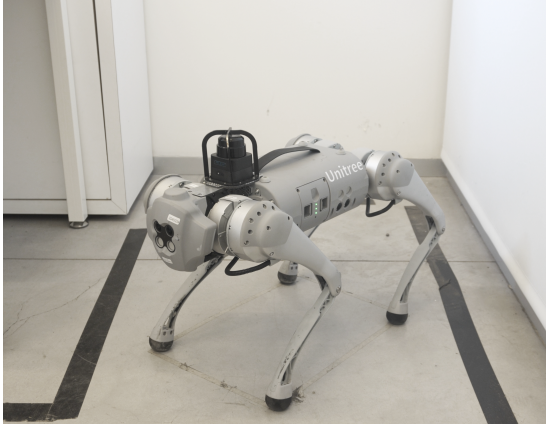
Figure 3: Unitree Go1 quadruped robot used in the experiment.
