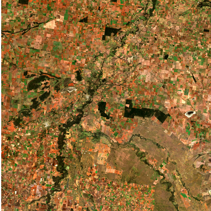
Fig. 6.2 RGB composite image where the B4, B3, and B2 bands regulate the intensities of the Red, Green, and Blue channels, respectively.
