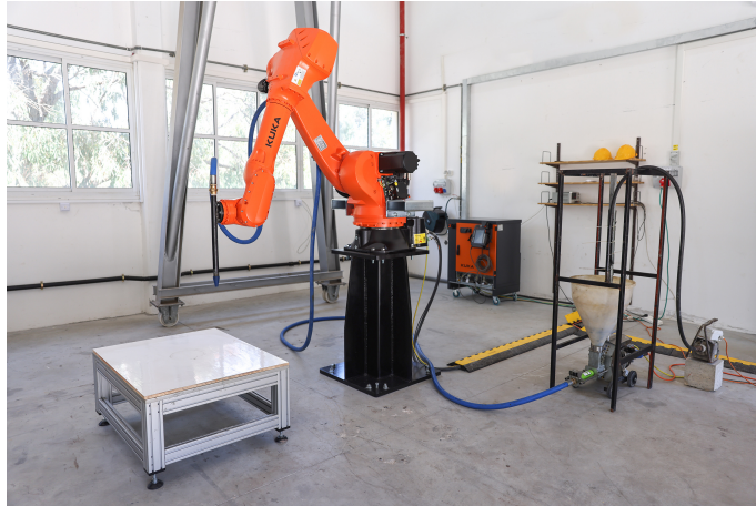
Figure 4: Robotic cell setup for 3D printing of clayey soils, featuring an industrial robotic arm, mortar pump, and concrete vibrator.
