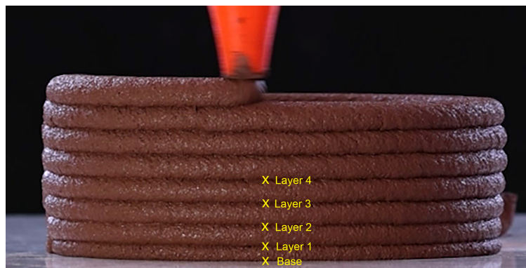
Figure 15: Digital Image Correlation (DIC) analysis illustrating based on layers strain during the 3D printing process.
