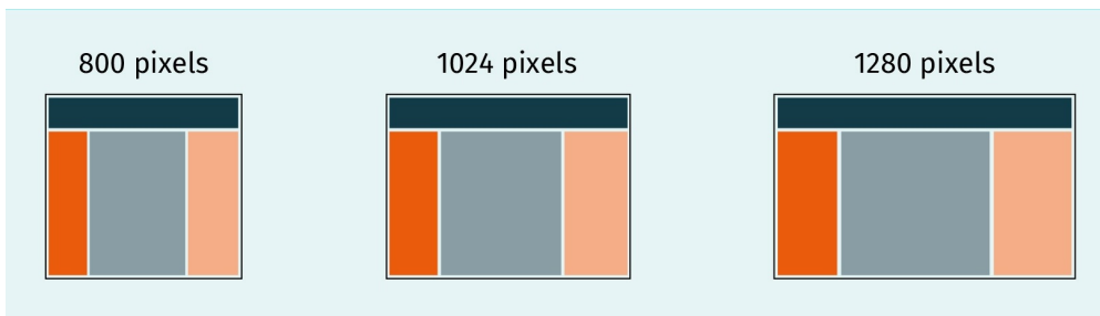
Figure 55: Fluid Layouts Always Assume the Same Relative Dimensions with Respect to Their Environment
