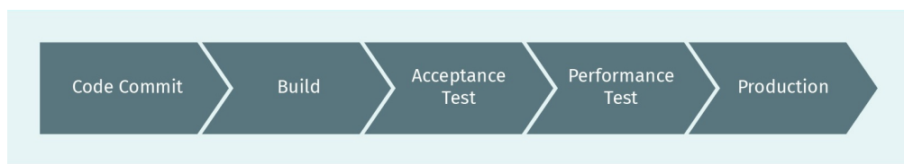
Figure 22: Continuous Delivery Pipeline
