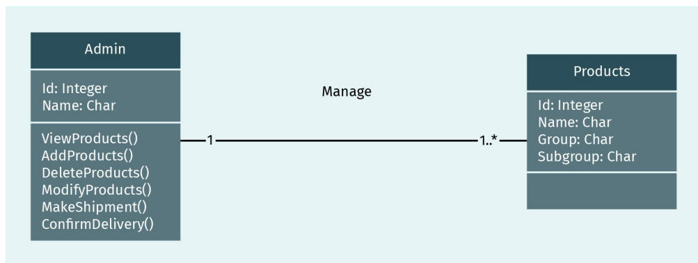
Figure 9: UML Class Diagram for an Online Shop
