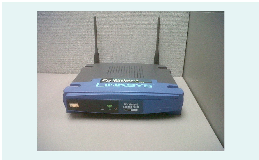
Figure 59: Wireless Access Point
