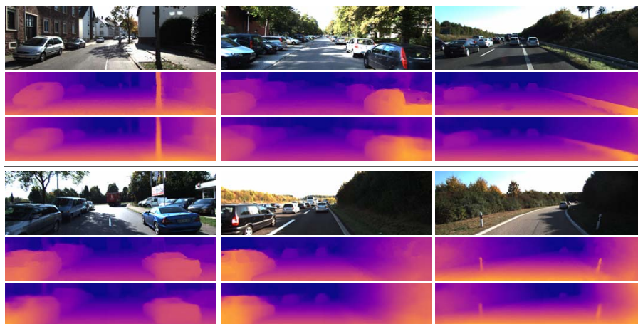
Fig. 3. Qualitative results of our DABC model on the KITTI validation dataset: original color images (top row), ground truth depth maps (center), and predicted depth maps (bottom row). Color indicates depth (purple is far, yellow is close).
