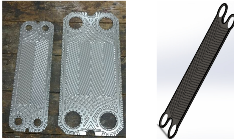
Figure 2 - a) Heat Exchanger Plate Samples, b) Heat Exchanger Plate CAD Model
