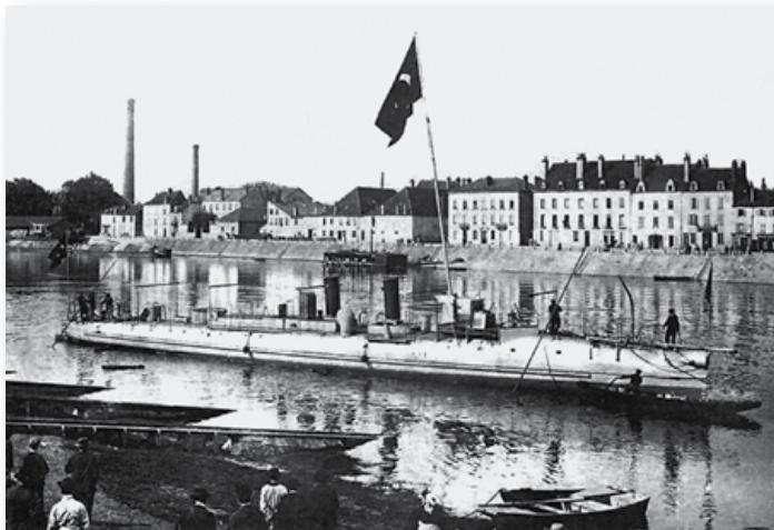
One of the Demirhisar class torpedo boats after being launched at the yard of Schneider & Cie at Chalon-sur-Saône.
