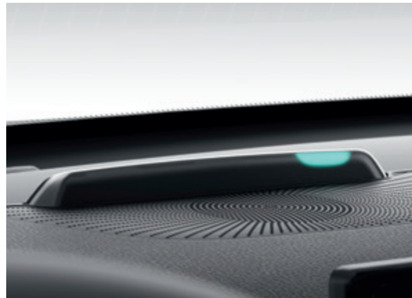
Charging indicator. Keep track of your charging status with the handy charging indicator. Located within the speaker grille in the middle of the dashboard (and easily visible even from outside the car), the indicator's three LED lights activate as you plug in to charge and keep you informed of the charging status and battery level.
