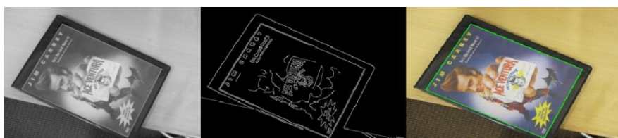
Fig. 6: Canny edge-detection function for a DVD cover detection, left side is the grey-scaled image, next to it is edges extracted on it; the right side is contour as a rectangle shape
